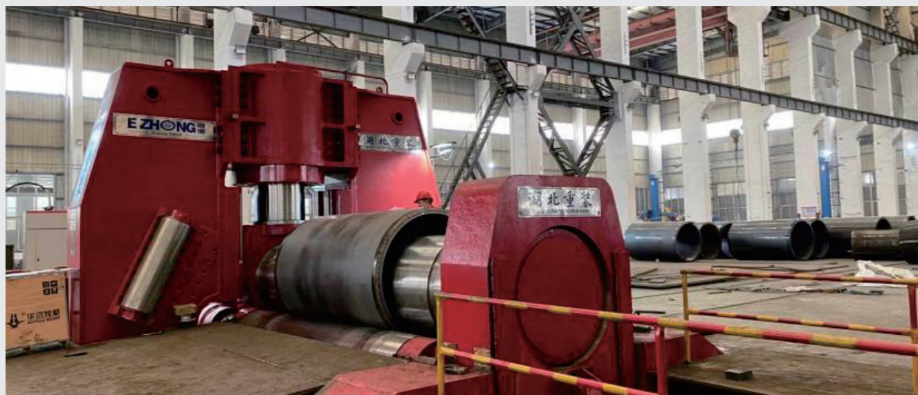
EZW11S-200x4000重型卷板机 EZW11S-200 x 4000 heavy duty plate rolling machine
